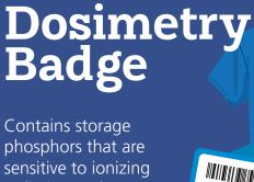
radiation and are used for monitoring radiation exposure to R.T.s.
